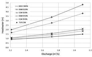
**Figure 3c** – Box culvert test results for B=1.2 m, D=0.6 m and outlet control.
