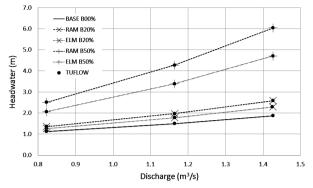
**Figure 3a** – Pipe culvert test results for D=0.75 m and outlet control.
