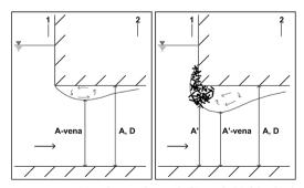
Figure 2 – (a) Clear culvert (left) and (b) blocked culvert (right).
